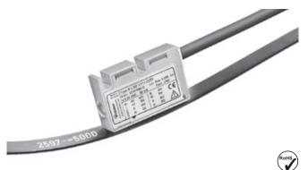
The non-contact incremental magnetic linear measurement system LI20 / B1 - made up of the sensor head LI20 and of the magnetic band B1 - reaches a resolution up to 10  $\mu$ m with a maximum distance of 1 mm between the sensor and the band.
