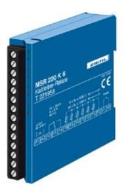
The MSR 220 K 6 monitors up to 6 PTC-reseitor sets with up to 6 PTCs each at the same time. If a temperature rise occurs in one set, the output relay releases and LEDs show the overheated sensor.
