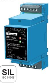
PTC-relay for the application as a protection device against inadmissible heating up at electrical equipment in areas with explosive gases (zones 1 and 2) and areas with combustible dust (21 an 22), e.g. for direct temperature-monitoring of explosion-proof motors EEx e and EEx d.
